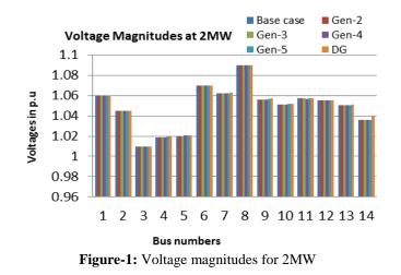
When the generators-3, 4 & 5 are rescheduled by 2MW, the available voltage in buses 1, 2, 3, 6, 8,12 are constant, while in the remaining buses 4, 5, 7, 9, 10, 11, 13, 14 the voltage variation is very small are shown
