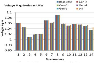
Figure-2: Voltage magnitudes for 4MW
